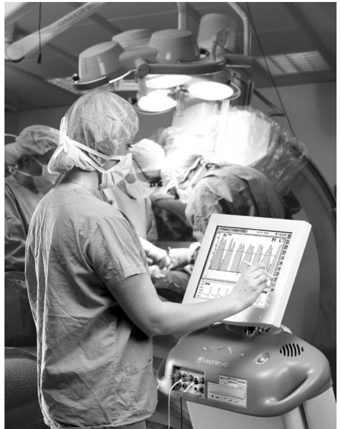
Fig. 8. A computer-based transit time flowmeter, Medi-Stim VeriQ.
